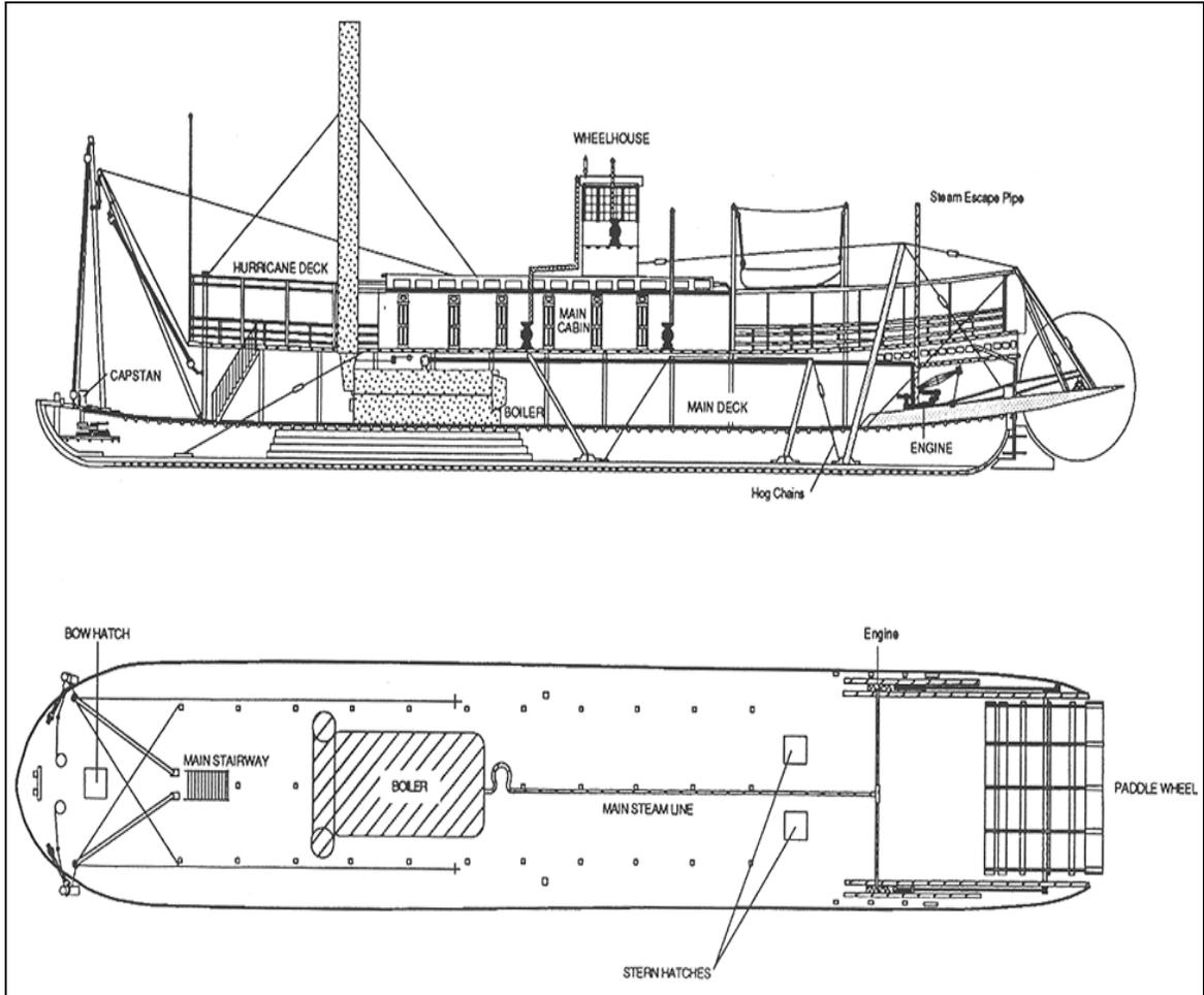
**Figure 19. Plan and profile view of a typical western rivers sternwheeler (after Petsche 1974).**
