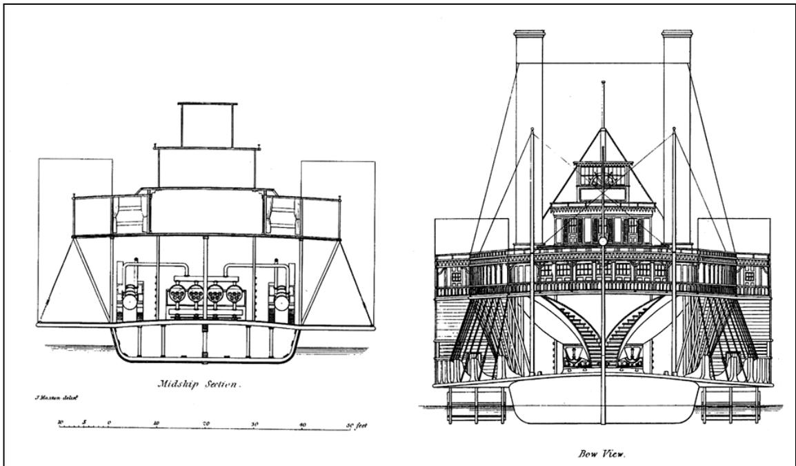
Figure 17. Midship section and bow view of a typical western rivers steamboat of the 1850s (as presented in Hunter 1949: 18).
