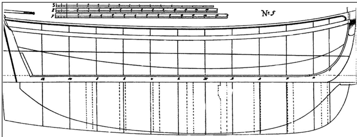
**Figure 9. Hull lines of a 34-foot longboat (as presented in Chapman 1768:58).**
