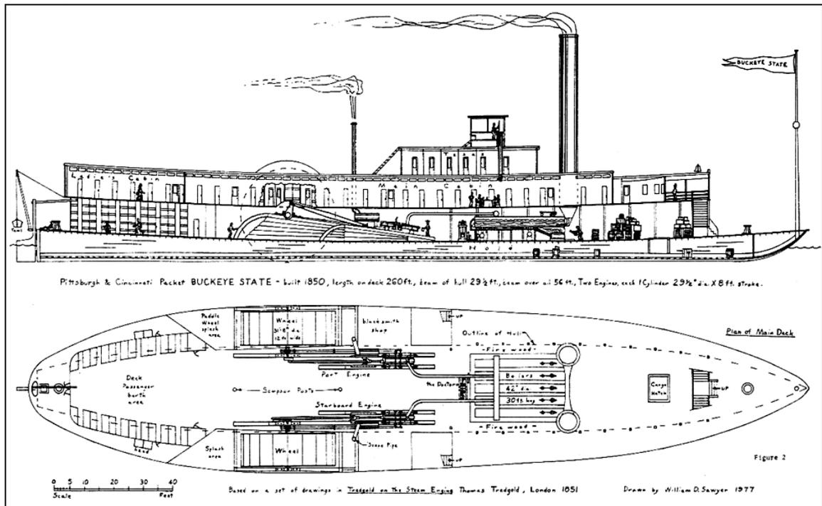
Figure 18. Plan and profile of a typical western rivers sidewheel steamboat of the 1850s (as presented in Sawyer 1979:74).
