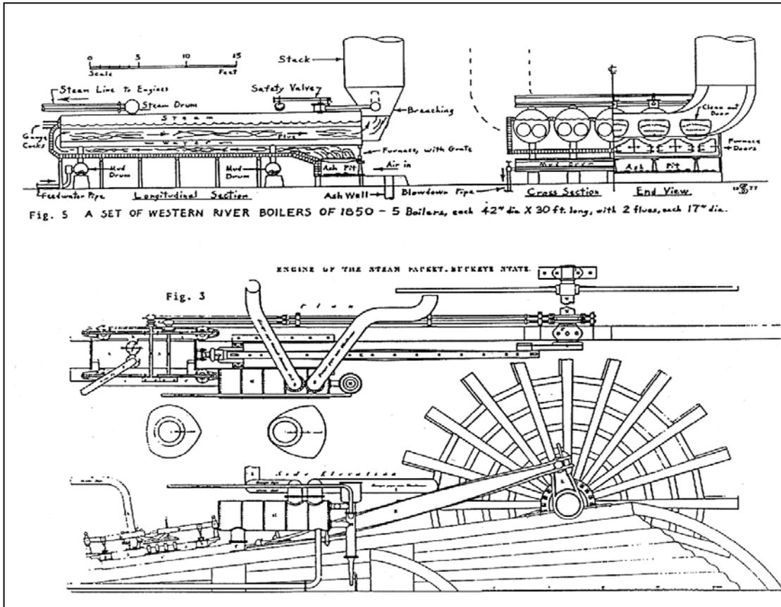
**Figure 16. Illustration of an 1850s steamboat boiler and engine (as presented in Sawyer 1978:75).**
