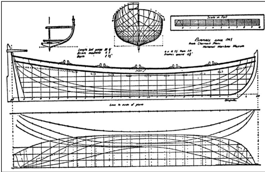
**Figure 10. Hull lines of a 1700–1750 pinnace (as presented in Chappelle 1951:23).**
