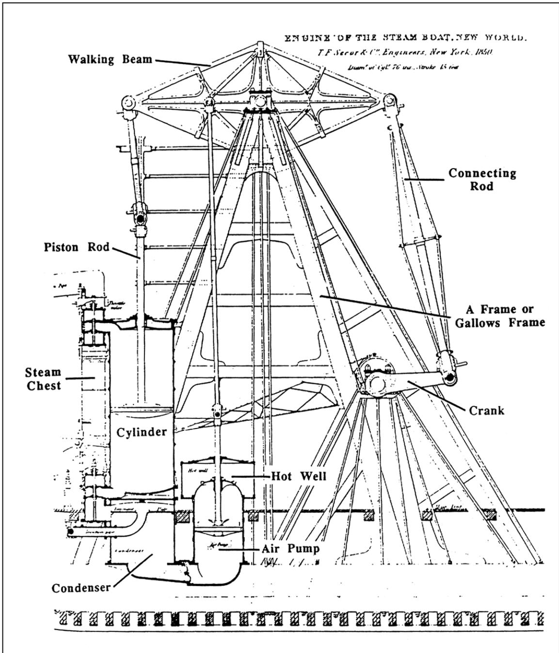
Figure 14. Major components of a mid-nineteenth century eastern seaboard low-pressure walking beam engine (as presented in Pearson et al. 1994).
