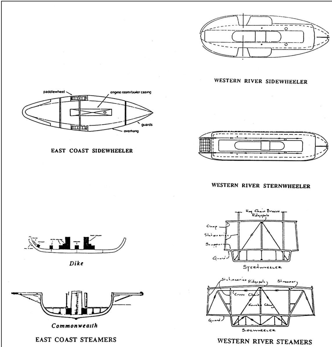
Figure 13. Comparison of hull shapes (top), and hull cross sections (bottom) of eastern seaboard and western river steamboats (as presented in Pearson et al. 1993)
