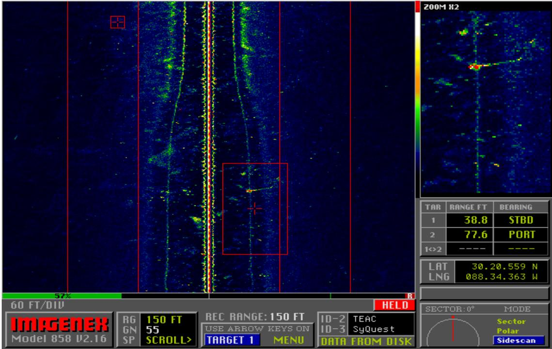
Figure 26 - Side Scan Sonar Image of Buoy Mooring
