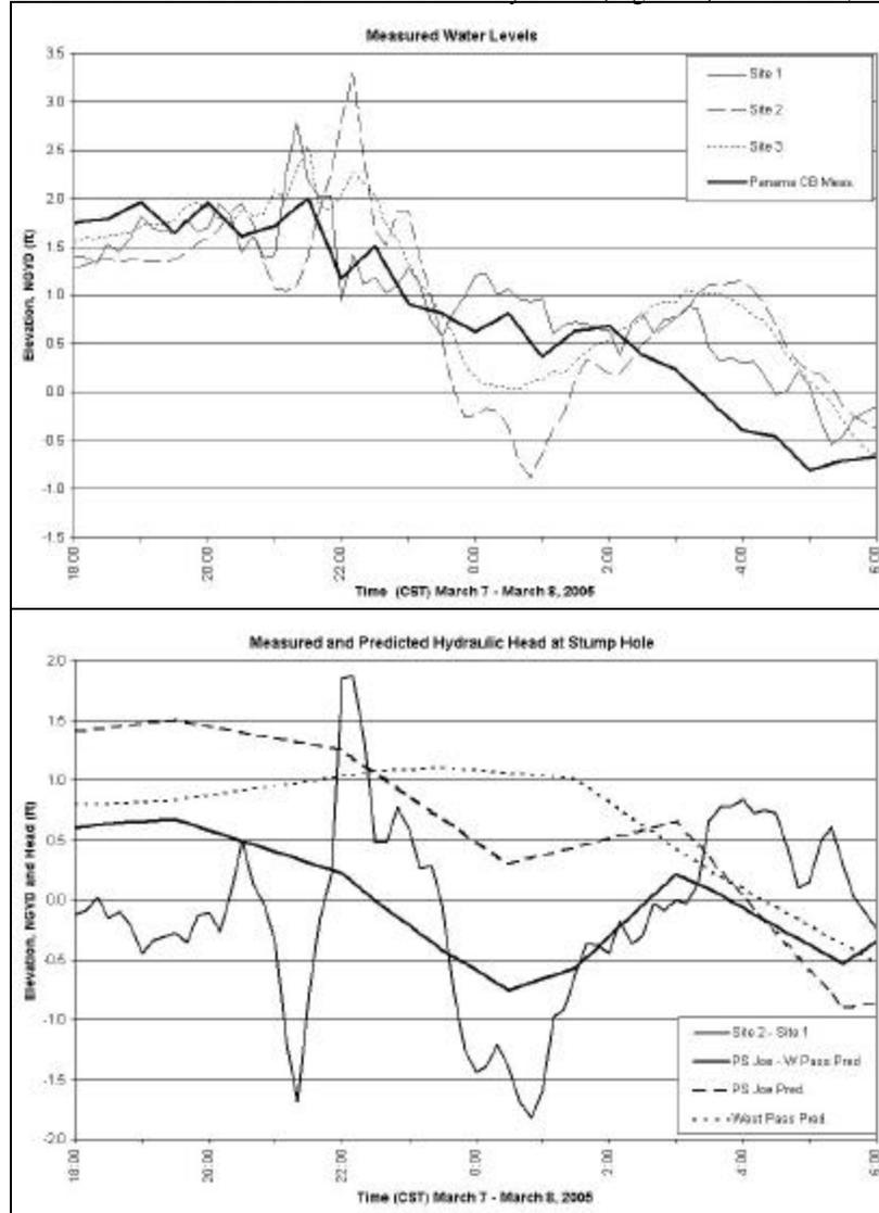
**Figure 7 - (a) Measured water levels during the frontal passage; (b) the measured and predicted hydraulic head during the frontal passage.**
