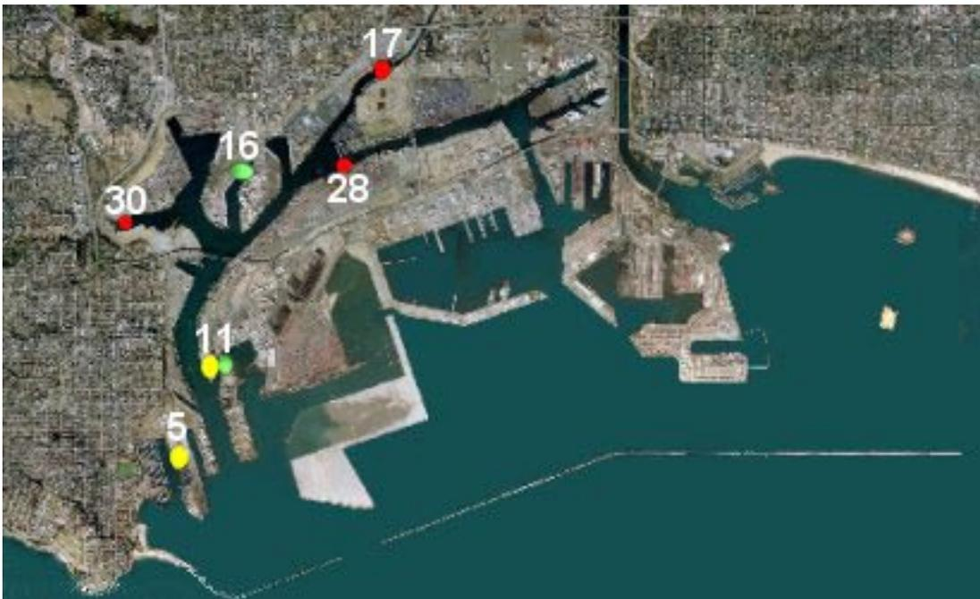
Figure 20. Location of Sites Showing Significant Degradation with Crest Loss (yellow if it occurs at + 7.5 ft, red if at + 10 ft) and Improvement with Crest Repair (green)
