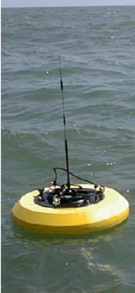
Fig. 6. NSI Wave Sentry Buoy
