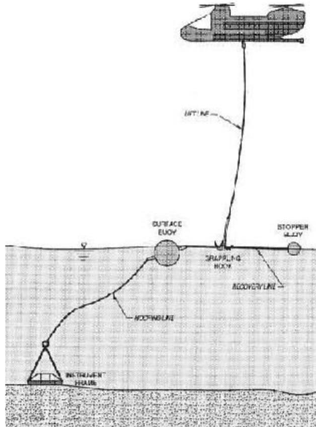
Fig. 5. Release and recovery of instruments with Chinook
