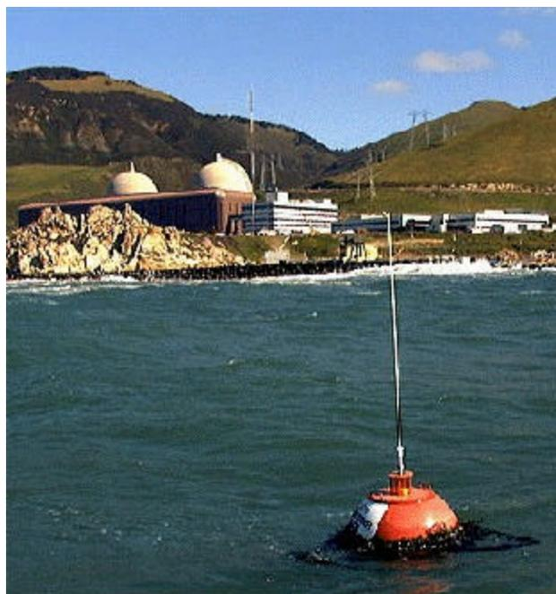
Fig. 3. Waverider (TM) buoy at Diablo Canyon, CA.
